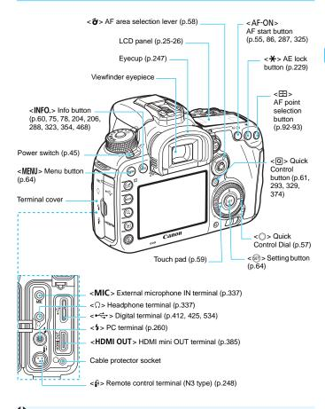
When connecting the interface cable to a digital terminal, also use the provided cable protector (p.34).
