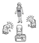
You can divide the slave units into two firing groups, A and B, and adjust the lighting balance (flash ratio) for shooting. The exposure is controlled automatically so that the total flash output of firing groups A and B results in the standard exposure.
